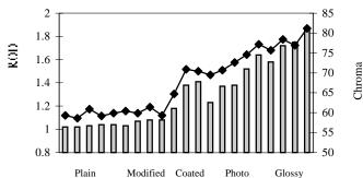
Figure 6. Influence of the media type on optical density. The Chroma is the line plot and ROD the bar chart.
