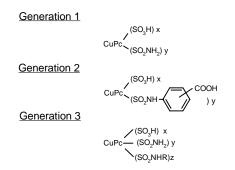
Figure 3. Structurally Modified Direct dyes for ink jet
