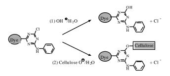
Figure 9. (1) Hydrolysis of a reactive dye. (2) Fixation to cellulose.
