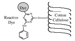
Figure 4. A covalently bound fibre reactive dye
