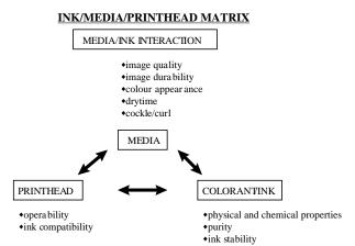
Figure 1. Interaction of the three key components involved in producing an ink-jet image.
